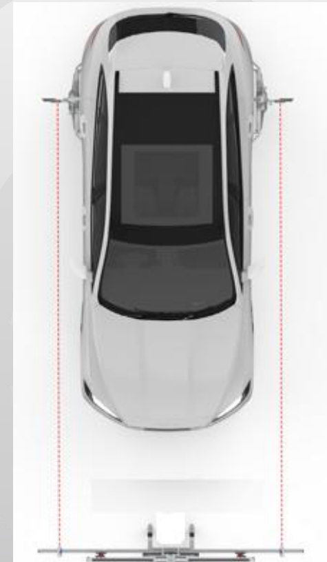
Laser range finders at both sides determine that the frame is parallel to the vehicle axle.
