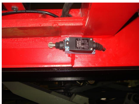
Picture 23 (main lift up limit switch)
