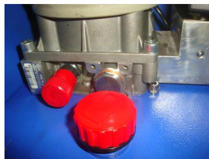
Picture 31 (oil tank)
