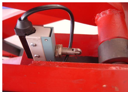
Picture 24 (second lift up limit switch)
