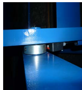
Picture 19 position to fix the limit switch
