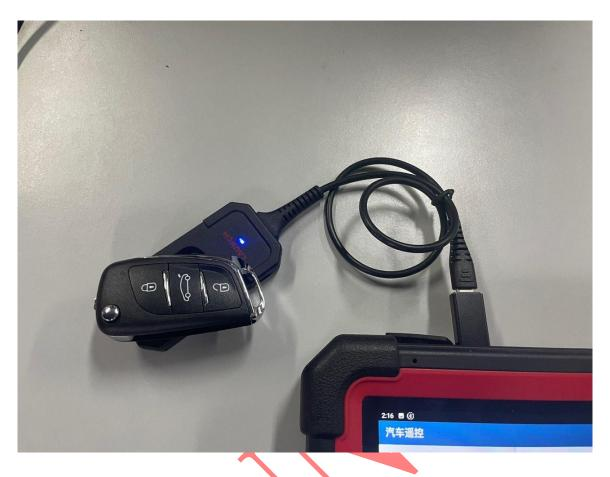
2. For car models without electronic keys, enter [Set type of wireless remote] to generate the corresponding key.
