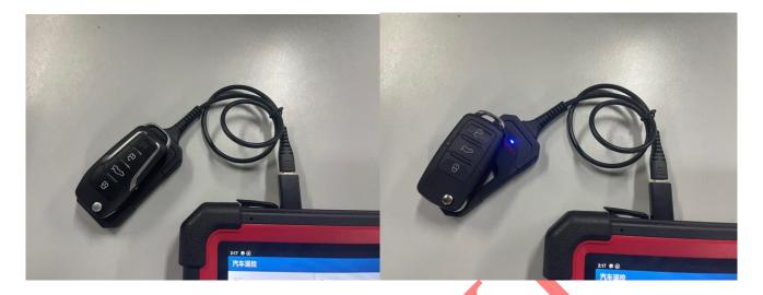
3. After the remote control is successfully generated, enter the [Set type of super chip] menu to generate the corresponding key chip.
