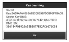
12) Place a new key close to vehicle coil, tap OK, and wait for the key to generate.
