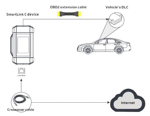
4. After a successful network connection, the SmartLink C screen displays prompt information asking whether to enter the super remote diagnostic mode. Tap Yes, the system will automatically read the vehicle information and connect to the remote diagnosis server.
