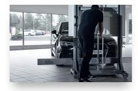
Adjust the upper reference panel to the height in accordance with manufacturer specifications (1.85 m for transporter). Exact positioning is made easier with the help of spring relief.
