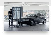
The calibration rig is mounted on a trolley making it easy to move and adjust.
