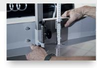
Lift or lower the panel for a parallel alignment by means of a lever.
