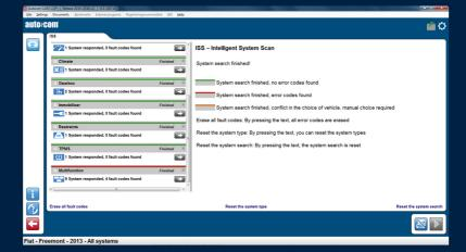
With ISS, your fault search process can be shortened considerably. Start up the ISS function and it will analyse all the controls in the vehicle. Upon completion of the scan, you will be able to see where the error codes are through the color codes of the control system. You can then continue to the various systems to implement a more advanced troubleshooting using real-time data, adjustments and adaptations.
