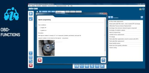
Under the OBD function tab in the software, you will see the different options for adjustments and adaptations without having the vehicle present before you. It is especially useful when looking for functions that you do not know which system it is classified under. As an example, key programming can be found under system immobilizer in some models while for some brands it can be found in another system.
